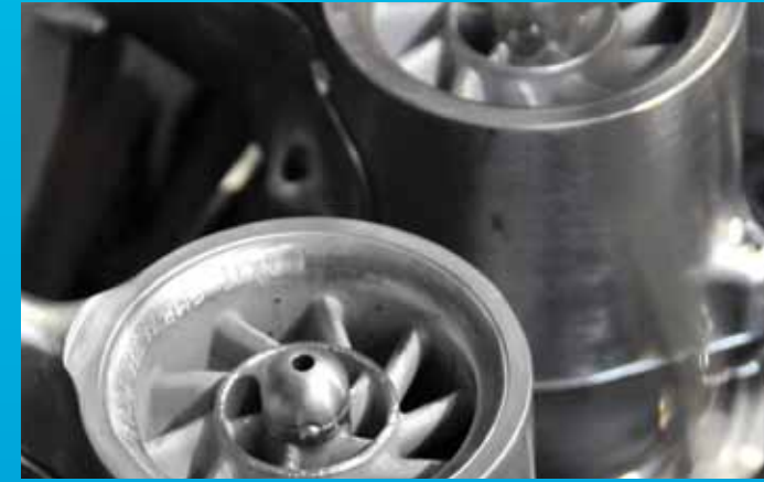
Premixers with double counter-rotating swirler.
