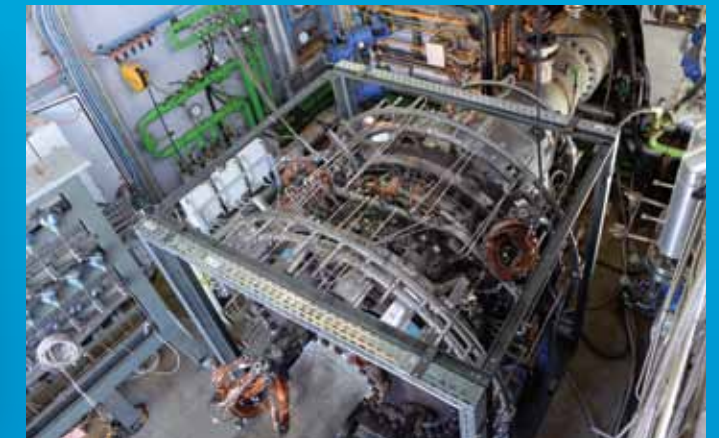
Full scale combustion vessel for full-annular-rig test.
